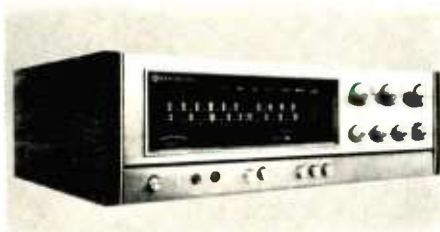
FIG. 5—KENWOOD'S KR-6340. One of many models using DSD circuit in stereo decoding section. Unit is a Quadraphonic receiver.
