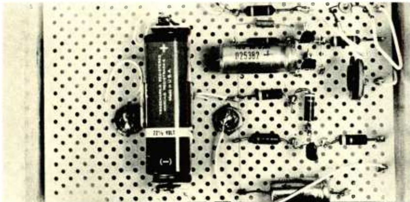
INTERIOR VIEW OF A BLITZMETER. This model uses point-to-point wiring on a perforated board mounted directly on the terminals of the panel meter.
