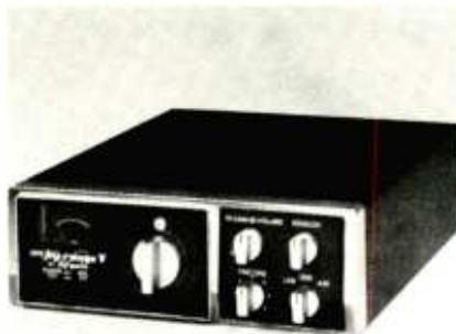
THE HY-RANGE V is a synthesizer AM/SSB rig whose circuitry is more complex.
