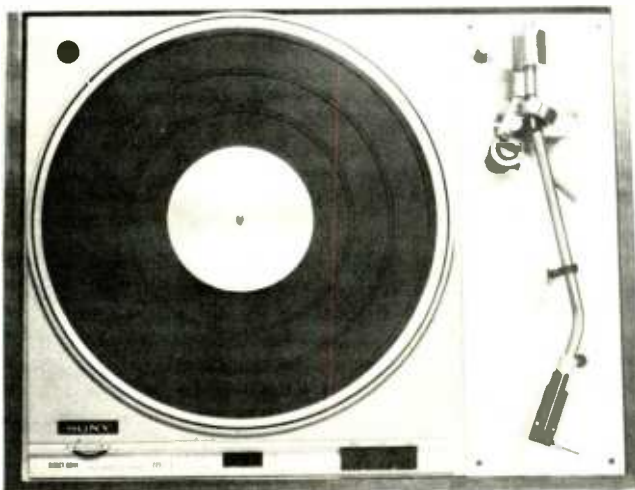
FIG. 9—TOP VIEW OF SONY PS-2251 turntable/toner arm assembly.
