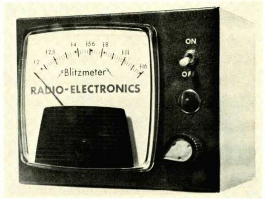
ONE VERSION OF THE BLITZMETER. This model uses rectangular meter and point-to-point wiring on perforated board. The other type uses a PC board and an edgewise panel meter.
